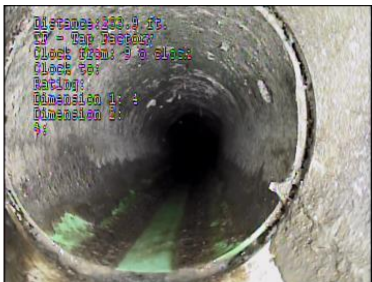
SITE 16: Separation of pipe connection between main PVC Sewer Pipe (8 inch) and PVC house connection pipe (3 inch) between Garfield SSMH-10 and Wilson SSMH-5. Separation 232 feet west of Garfield SSMH-10.
