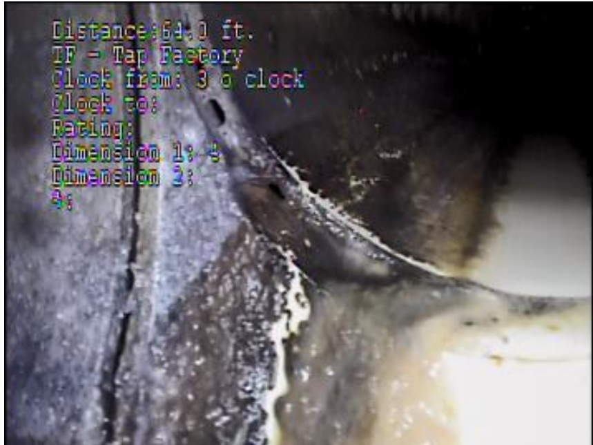
SITE 8: Separation of pipe connection between main PVC Sewer Pipe (8 inch) and PVC house connection pipe (3 inch) under a side street. 64 feet north of Sumas Ave SSMH-2.
